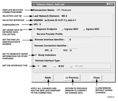
Figure 791-7. Add Leaf Window - Configure Endpoint
